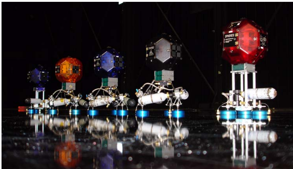
Figure 6.3 Five satellite TPF maneuvers at the MSFC Flat Floor
